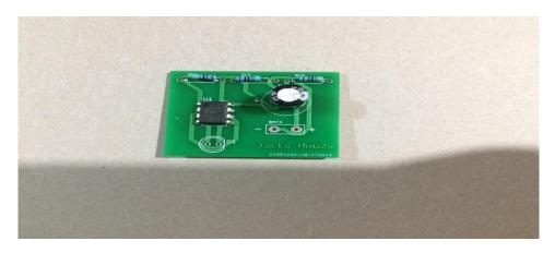
3. Place the resistors in their correct hole then solder in place.
