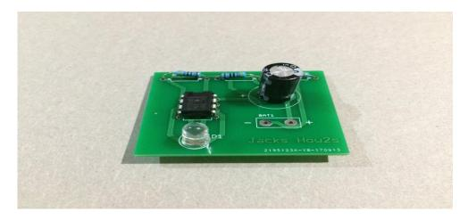
4. Place the Led in the socket labelled **D1** with the flat side of the led corresponding with the flat side on the PCB again solder the legs in place.
