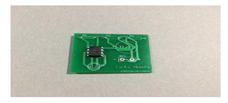
1. Start by placing the 555 timer ic into the U1 space with the notch on the ic corresponding to the notch on the PCB and fix in place with solder.
