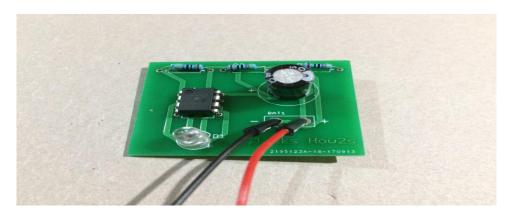
5. Lastly connect the red wire to the + hole of the PCB and the black wire to the -hole of the PCB solder the wires in place.
