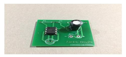
2. Place the 33uF capacitor into the C1 socket making sure that the longer leg of the capacitor is in the + hole and the shorter one in the other, then fix in place with solder.
