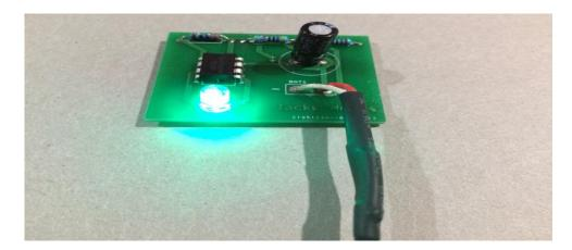
6 Connect a 9 Volt battery to the battery clip and the LED should flash/strobe! If not please read the instructions and check the position of the components.
