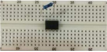
2. Place one 10k resistor from pin 8 of the ic to pin 7,
