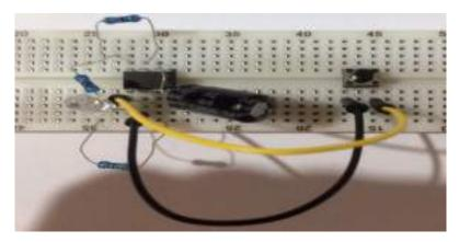
6.Now connect one leg of the push button to pin 2 and the other leg to pin 1,
