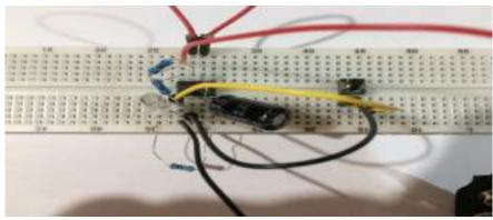
7.Place a jumper wire connecting pin 6 and 7 together,
