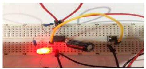
8.Lastly connect the black wire of the battery to pin 1 and the red wire to pin 8 connect the battery and press the button! The light should turn on for approx 12 seconds, if not check the component position using the following references.
