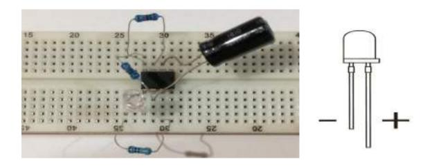
5.Connect the negative leg of the led to pin 1 of the ic and place the 330 ohm resistor from pin 3 to the positive leg.
