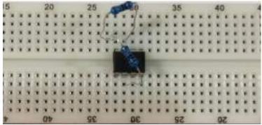
3. Place another 10k resistor from pin 8 of the ic to pin 2,
